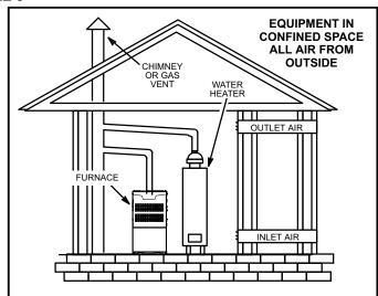
NOTE - Each air duct opening shall have a free area of at least one square inch (645 mm²) per 2,000 Btu (.59 kW) per hour of the total input rating of all equipment in the enclosure. If the equipment room is located against an outside wall and the air openings communicate directly with the outdoors, each opening shall have a free area of at least one square inch (645 mm²) per 4,000 Btu (1.17 kW) per hour of the total input rating of all other equipment in the enclosure.
